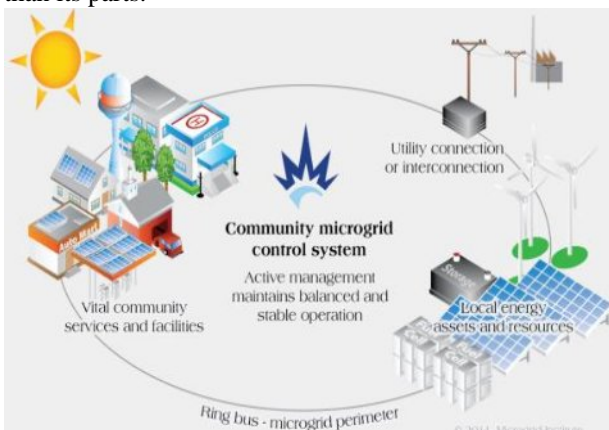
Fig.1 Microgrids Combine Various Distributed Energy Resources (DER)
